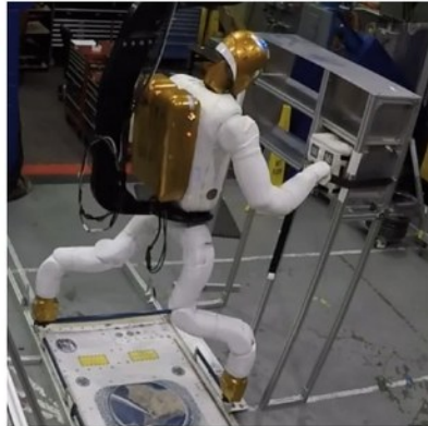
d) Unbuckling a strap holding a CTB
