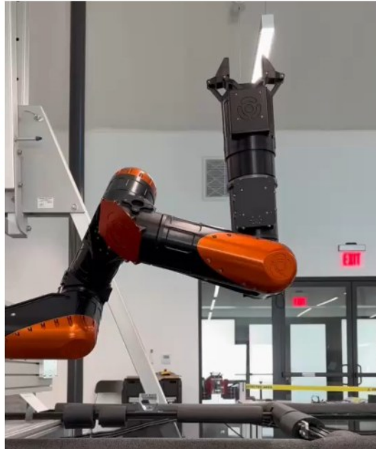
Compliance control enables collaborative tasks with any RLR
