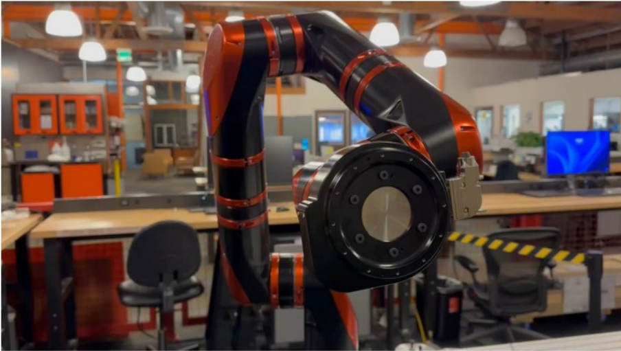
Compliance control enables collaborative tasks with any RLR
